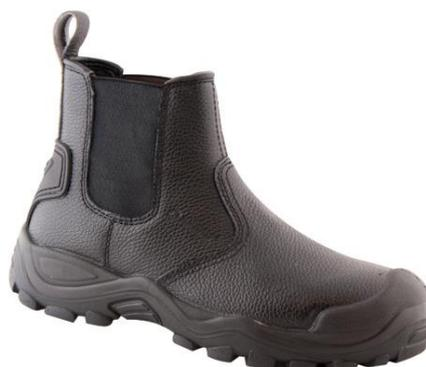
PU2D/ rubber sole is antiwriting, antistatic, resistant to oils and fuels and contact heat up to 300°C. Shoes with increased protection in heel area and with tab for easier putting on. In ankle area are safety side inserts from the combination of rubber and textile which are determined for quick putting off in the case of scale penetration to the shoes. This shoes are suitable for use at foundry industry.
