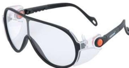
Protective glasses with black nylon frame and temples with orange ratchet knob. They suit perfectly to every user because of adjustable temples length and tilt. Exceptionally wide field of vision offers maximum coverage and protect against UV radiation. They are anti-fogging, anti-scratching and resistant to low-energy shocks (up to 45 m/s) at extreme temperatures (-5 °C - +55 °C). These glasses are fitted with integrated side shields and provide high-level protection.
